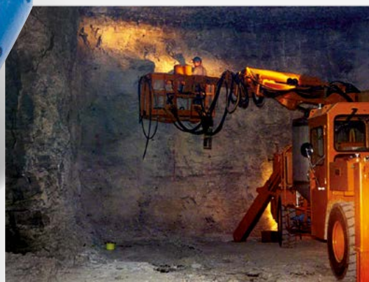
Mine vehicle with horizontal swiveling and telescoping platform, whose arm is moved by a WD-H 0300 slew drive
